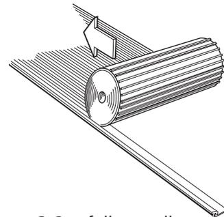
**3** Carefully re-roll the mat leaving snap track in position.
