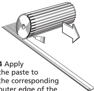
**4** Apply the paste to the corresponding outer edge of the contacting bar and bar edges - pasting approximately 1 metre sections at a time. Slowly unroll the pasted mat section aligning and joining to snap track on floor (as indicated by the shaded area).
