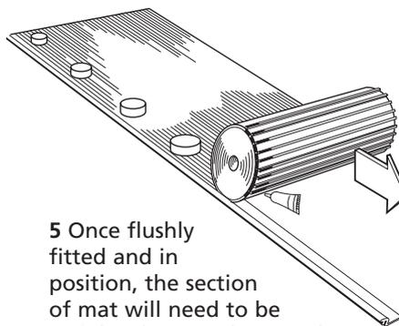
**5** Once flushly fitted and in position, the section of mat will need to be weighted at evenly spaced intervals while the paste bonds. **DO NOT** disturb joints for 30 minutes.
