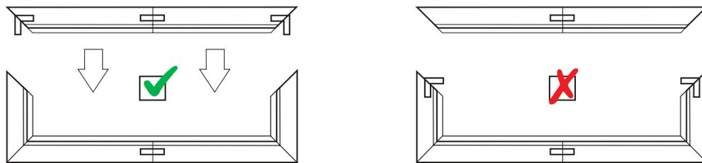
Fixing to the floor - It is recommended that the aluminium frame is fixed to the floor, using the screws and rawl plugs provided. The countersunk holes in the frame can be used to mark the hole positions on the floor. The holes should be drilled 6mm in diameter and 36mm deep to suit the screws and plugs provided.
