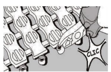
When fitting 'B' cut off spacing and click together
