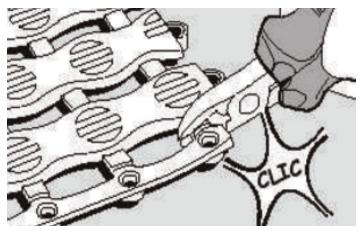
3) Edging ramps can be attached (on parallel sides only) When fitting 'A' click together as in step one
