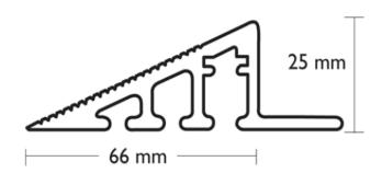
3) When the aluminum ramp meets the side of the tile, the extra tag can be removed by simply cutting it.
